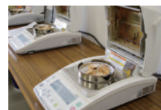
Graph of Wood Chip Moisture Content Measurement and MOC63u Electronic Moisture Analyzer
